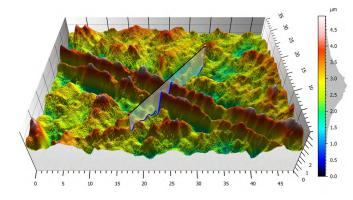
**3D** topography of a polished solder surface reconstructed from SEM images using SMILE VIEW<sup>™</sup> Map software
